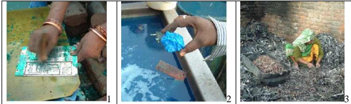
Figure 5: The extraction of copper from printed wiring boards (PWBs)
